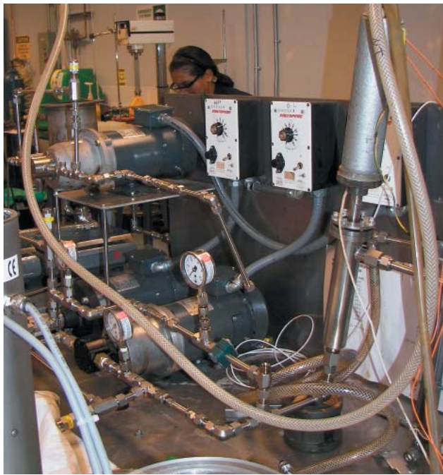
SulphCo says that the continuous flow-through unit pictured above can mimic the Sonocracking™ process more realistically than its initial oil sample batch testing equipment.
